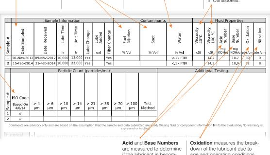
Acid and Base Numbers are measured to determine if the lubricant is becoming acidic. A lubricant that becomes too acidic can cause corrosion to internal engine components. Note that acid and base numbers do not begin at zero. Oxidation measures the breakdown of the lubricant due to age and operating conditions. Nitration occurs when nitrogen oxides react with the lubricant, causing deposit formation and an increase in viscosity. Note that oxidation and nitration readings do not begin at zero.
