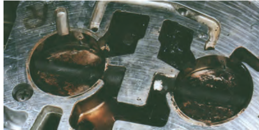
Picture J - Carburetor plates before P.i. treatment
