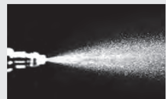
Injector spray pattern after P.i. treatment.
