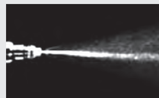
Injector spray pattern before P.i. treatment.
